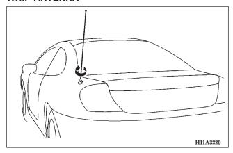
To remove the whip antenna, turn it counterclockwise.
